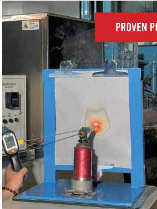
FireKover™ has passed multiple rigorous evaluations, including flame-resistance, gas-toxicity, and heat-release-rate tests.
